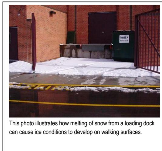
This photo illustrates how melting of snow from a loading dock can cause ice conditions to develop on walking surfaces.
