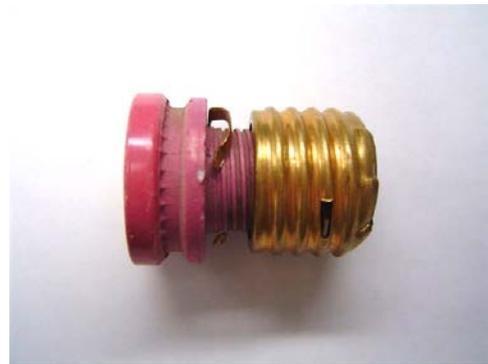
Screw the Fustat® into the base adapter (as shown above), and then screw the combined assembly into the socket on your electrical panel. The next time you unscrew this fuse, its base adapter will stay in place and will only accept the Fustat® fuse in the correct amp rating
