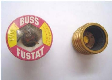
Fustat® fuses, (also called type S) as shown in the image above, are not interchangeable, meaning you cannot install a 20-amp fuse into a 15-amp base. The base adapter on the right screws into any fuse socket
